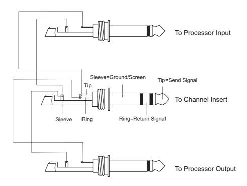
Y-Stereo lead for insert Connection
