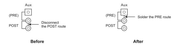
Modification on mono and stereo channels
