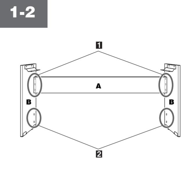
**1 Loosen the screws attached to stand part A.**
